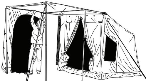
Note: For easy set-up, lower down the 1.9m poles before zip on the panels.
