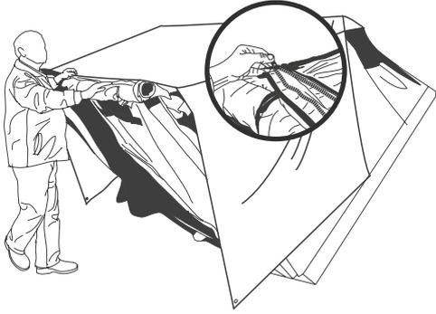
2. Place the 1.7m poles on each side to create spacing and secure with guy ropes as shown.
