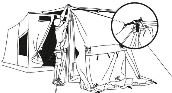
4. Peg at all base peg points and set up support poles. Extend all guy ropes, peg and secure.
