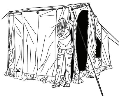
3. Zip the sides of the Front Panel to the sides of the Side Panels and secure velcro tabs.
